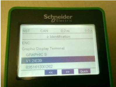
3. Then Push the button "ENTER" for 5s, until the graphic keypad displays again the menu "2.IDENTIFICATION".
